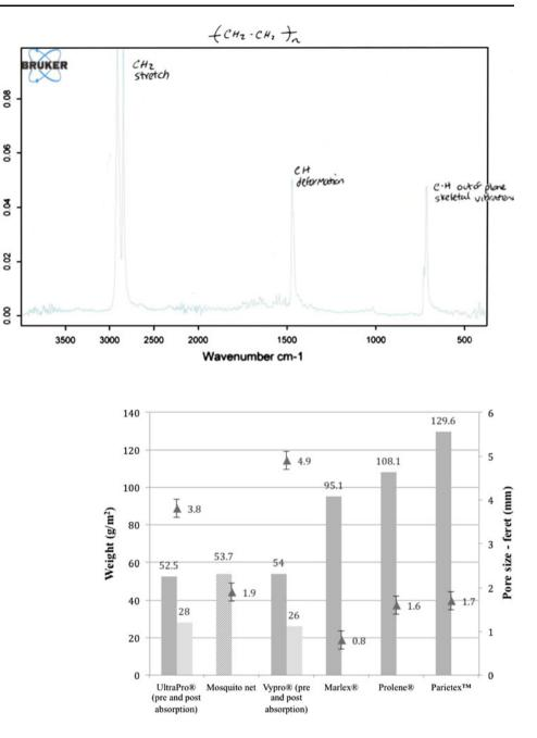
Fig. 3 Weight and pore size of mosquito net compared to commercial hernia meshes (weight displayed as *columns* and pre and post absorption weights shown where applicable. Mean pore sizes displayed as a *scatter plot* with the SEM shown)
