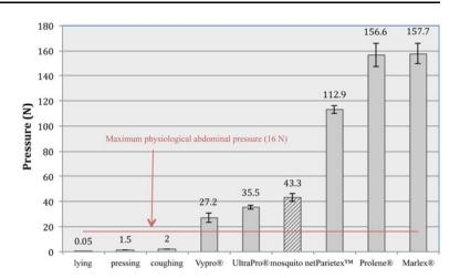
maximum tensile strengths, subsequent tearing forces, maximum bursting force, or percentage deformation at 16 N between mosquito net and the lightweight (Vypro and UltraPro) commercial meshes.
