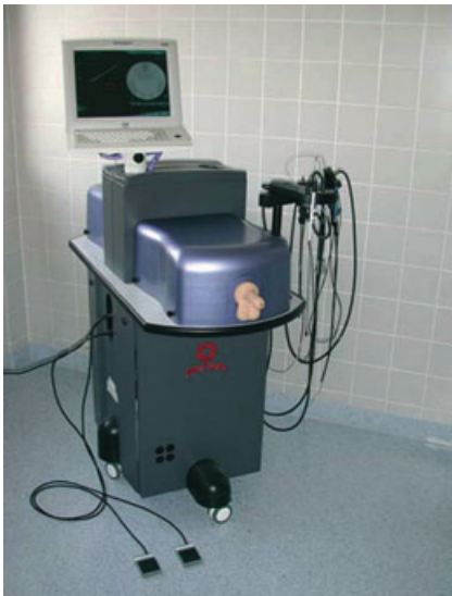
FIG. 3. Uro Mentor system (Symbionix) for ureterorenoscopy.
